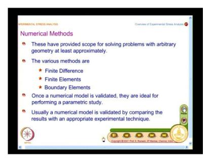
So, what you find here is, even though you have methods, which provide the conceptual understanding if I go for arbitrary shape, numerical methods, come they handling. And you are able to get the solution at least approximately, for arbitrary geometry, so that is where you find the numerical methods very attractive.
