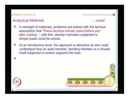
And what you find here is, so one of the basic assumption is plane sections remain plane before and after loading. And with this what we are solve? We are solved at large number of problems, which are slender in nature, very very it important, suppose I take a plate and then, stretch it like this, I have no problem. Suppose, I put up hole their I cannot do it strength of materials, the moment I put a hole the assumption plane section remain plane before and after loading no longer exists.
