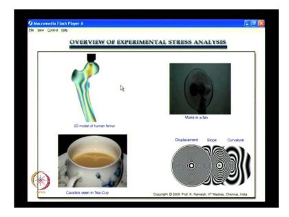
And these slide shows in nutshell what experimental analysis is all about. And what we see here is (Refer Slide Time: 00:26) stress patterns observed in a 2D model of a human femur. So you get stress information and stress analysis and you also get displacement information in stress analysis.
