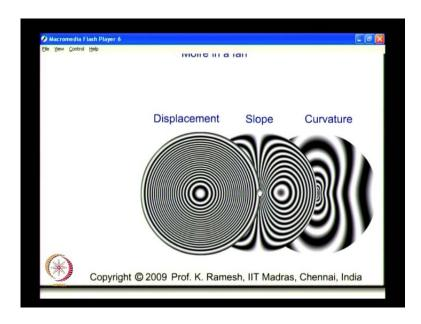
And what you find here is for a circular plate clamped at the boundary with a central load, you get the displacements. And you can also have the slope, you can also get curvature but, what you will have to appreciate here is, for each of this information, you need to use a specific optical arrangement. You would not get them in one shot but, you have to have effort to do that.
