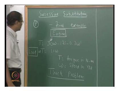
This is the problem number 7. We call it as the truck problem. Omega is the speed in rps and T is the torque in newton-meter. Torque T is given by 30 omega minus 175 minus 0.3 omega square and T equal to 11 omega. So, this is the engine characteristic and this is basically the load.
