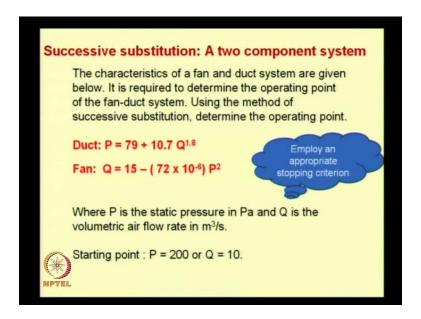
So, the equations for the duct and fan are given. So, I have already dictated this problem to you. So, there are two variables in this problem, one is P, which is the head, which is in for the pressure, which is in Pascal. So, the other one is the volumetric air flow rate, which is in meter cube per second. So, these two are (( )) by, these two by, the two respecting equations. Now, you want to solve and get the operating point.
