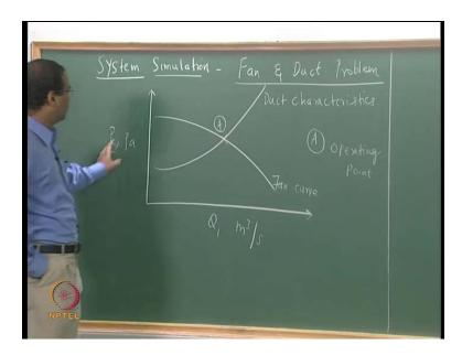
So, one is the duct characteristics where basically, the pressure rise, which is Q into 1 to the power 1 point, Q to the power of 1.8. This 1.8 is a consequence of the (()) equation, which gives you the head-loss flv square by 2gd. f itself is 0.182 Reynolds to the power minus 0.2. The 2 and minus 0.2, they combined to give 1.8. I have already discussed this in the last class.
