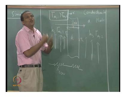
So, there is a slab, it has thickness x, thermal conductivity k, having steady state. So, here there is a heat transfer coefficient of h 1 and (()) temperature of T infinity 1, here we have a heat transfer coefficient of h 2, it is T infinity 2. So, this situation is typically encountered in heat exchange replication where there is a plate, which separates the two fluids. So, there is a heat transfer from one fluid to another fluid, let us say that.
