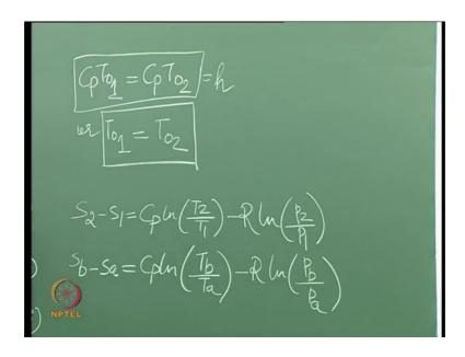
c p T 0 1 is equal to c p T 0 2 or T 0 1 is equal to T 0 2 what does this tell us, what this tells us is that the stagnation temperatures do not change across a shockwave. So, all the total temperatures do not change across a shockwave another thing that it tells us that C p this is nothing, but the enthalpy is not it now this is the total enthalpy. So, the enthalpy does not change across a total enthalpy does not change across a normal shockwave ok.
