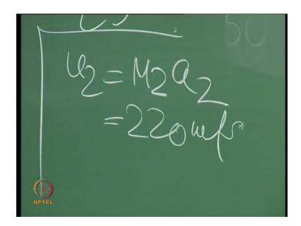
M 2 right. So, therefore, U 2 is equal to M 2 into a 2 and which we get as 220 meters per second. So, this is what is this is what we this is how we sort of finish this problem ok
