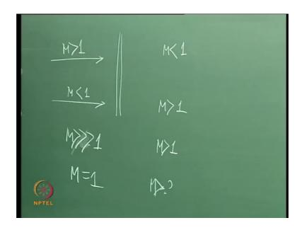
Is it that you have a very high supersonic flow now that really slows down here to subsonic and then we have a shockwave could it also be that I actually have a subsonic flow and it speeds up to very high speed supersonic flow and then we have a shockwave right or is it that you know we have a very very high mach number flow and slightly less mach number flow right both are supersonic by the way and we then have a shockwave and so on and so forth.
