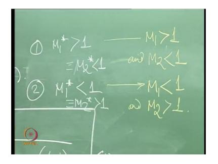
If M 1 star is greater than 1 then what we get from M 2 which means that this inference from here is that M 2 star is less than 1, that we can inform from B, but what can we infer from this again if M 1 star is a supersonic which means the corresponding M 1 is also supersonic. Now M 2 star is subsonic which means the star value is subsonic therefore, the corresponding actual value is also subsonic which means M 2 is subsonic
