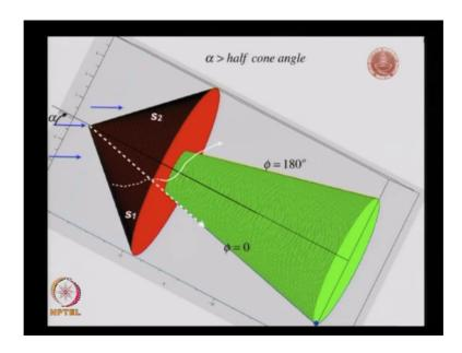
So, let us go to what happens if alpha? The angle of attack is greater than the half cone angle. What happens then? Right. So, we look at the same picture this alpha is just greater than the half cone angle it is the same picture. So, again we have to red line phi is 0 phi is 180 degrees and we have these streamlines. So, again the entropy change there is S 2 entropy change here is S 1 say and alright.
