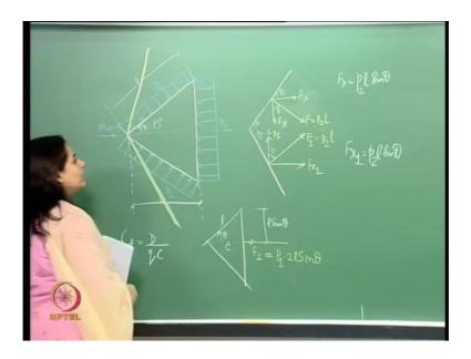
So, essentially if you have say and so, then this is theta. And so, I am going to call this length as 1. And we have an incoming mach number, we have this. So, basically, we have you know a wedge like this. So, the mach number is given the theta is given what we need to calculate is the drag coefficient for this wedge, and something else is also given. So, this distance is c.
