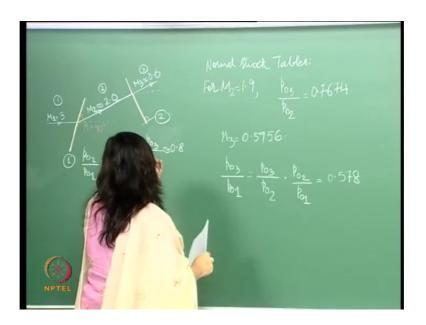
So, we will go to the a tables. So, using normal shock tables, from the tables using normal shock tables what we get is the stagnation is the yeah total pressures behind and in front of this normal shock. So, essentially, we get a ratio for p naught 3 by p naught 2 which comes out to be, right. Which comes out to be this. And it which is nearly 0.8 actually which is nearly 0.8, and M 3 comes out to be 0.5956 which is merely 0.6 nearly 0.6.
