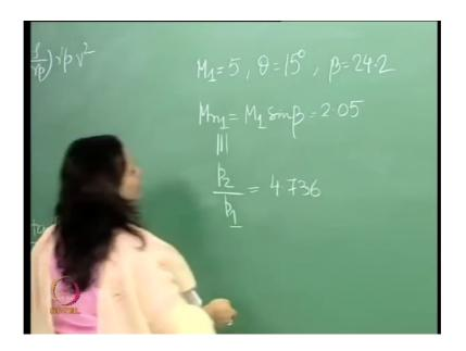
So, basically, we have a mach number. So, mach number is 5, and theta is equal to 15 degrees. So, using the charts theta beta m relationship, we get a beta in this case of 24.2. So, this is the incoming mach number, which we know theta is given. So, therefore, we find out the shock wave angle.
