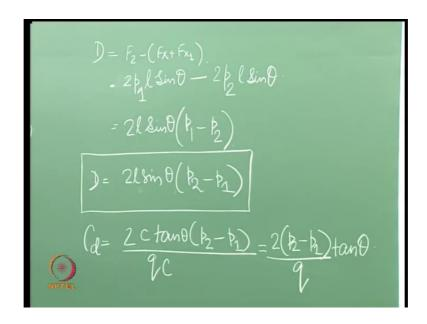
Now so, drag is basically the total forces in the horizontal direction the direction of the free stream. So, here now drag now that comes out to be so, if you look at, but it is important to see here, that this F these 2 this F x and F x 1 are in this direction F 2 is in the horizontal direction here, right. So, what it will be a you know, drag is basically
