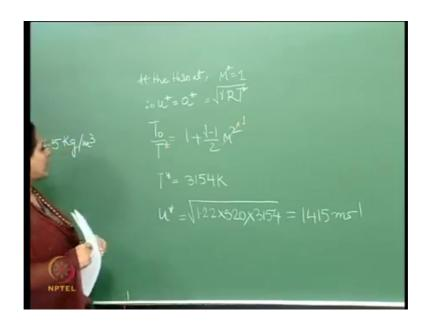
So, how do we do that? Now at the throat which is sonicson m star or mach number is 1. So, in at the throat so, therefore, u star is equal to A star, right. It is equal to the speed of sound right. So, which is again speed of sound using an equal to gamma R T, gamma R T and here because it is at the throat I can write this as T square, right. T star and a again gamma and R are constants which are known, I need to find out T star.
