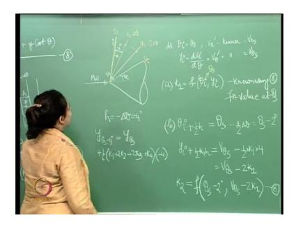
This is our cone right and we have a free stream which is coming in right and so, this is our shock wave. So, this is our shock wave. So, this is theta s and this is our surface which is theta c. So, what we doing here is essentially moving from theta s to theta c right we are moving from here to here.
