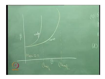
So, this is the shock wave angle and this is the cone angle or wedge angle over right. So, therefore, at the same Mach number right. So, we have say theta max here and let us call this as 1 and we have ok.
