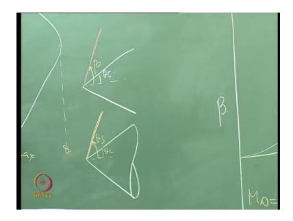
So, essentially you know the (Refer Time: 49:15) just plot this out. So, this was our 2D wedge this is our 2D wedge and so, then we have say a shock here and I am drawing the same thing say I am drawing the same thing over here for the cone and again I have say a shock wave and again this is theta c, this is theta s this is your beta right. See if you were look at these two pictures you know just to visualize this, this is in the plain of the board this here is in the plane of the board.
