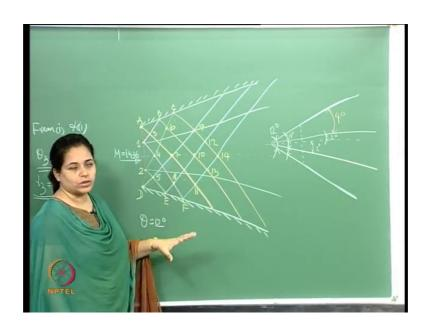
In this particular case is that we have in our channel like that we really need to be symmetric over here. So, I have a channel here like this we have a channel here like this and the and this is diverging by 12 degrees, it is diverging by 12 degrees and input mach number mach number coming in is 1 point say 4 3 6. So, how do we go about this? So, what we will do is if we.
