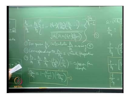
So far given diaphragm pressure ratio which is p 4 by p 1; so, you evaluate or calculate insulin shock strength right you can see from here directly.
