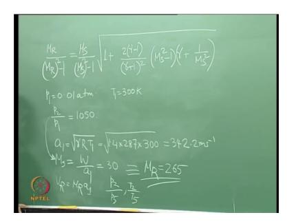
So, then what we get here is this is a kind of an expression that we get, ok. So, this is the relationship between the incident shock Mach wave and the reflected shock Mach wave. So, this is essentially the relationship between the incident shock Mach wave and the reflected shock Mach wave. So, if we know this then we shall have an estimate of this. So, let us sort of do a small problem based on this, and see what exactly we are talking about.
