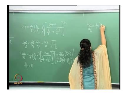
So, u p can be written as. Using three governing equations we can just come up with this, I am not doing the math which by this time hopefully you should be able to do that its preliminary elementary. So, this is more or less; this is the expression for u p and you can see we have written it out essentially in terms of the velocity of sound. In the driven section which is section 1 and the pressure drop of pressure ratios between the two sections.
