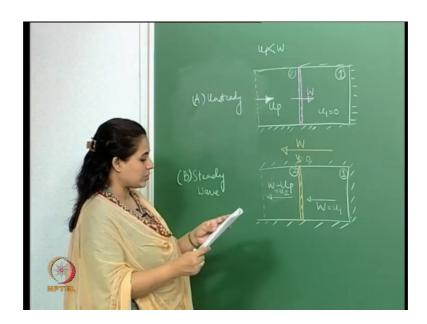
So, we have a shock which we have a shock which is travelling in a trough its right; this was is this is the unsteady shock wave travelling. If we have to convert this to the steady state case that we are most familiar with then all we will do is superimpose this flow with a velocity W in this direction.
