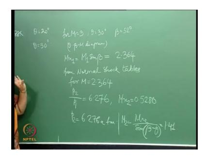
So, for this here again, so for M 1 equal to 3 and theta is equal to 30 degrees. So, from the theta beta M relationship from the theta beta M diagram we get so for this we get a beta this is from the, this is from the theta beta M diagram. So, from theta beta M diagram we get beta is 52 degrees. So, therefore, again right. So, the normal comprehend then comes out to be right.
