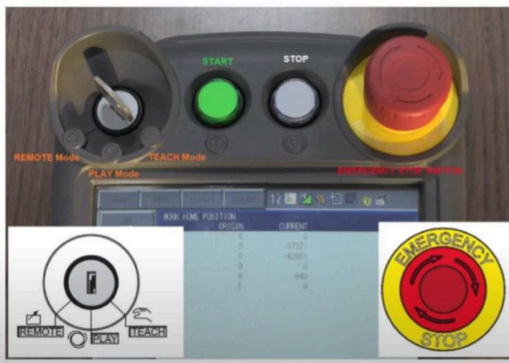
Switches on the Teachpendant of Yaskawa YRC 1000 Controller.
