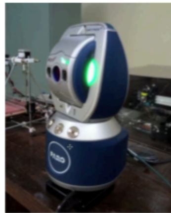
FARO laser tracker mounted on serial robot
