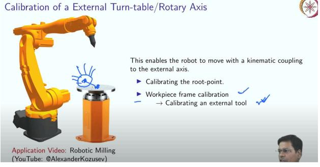
Now, let us move ahead. So, now we will be doing calibration of the external kinematic system. To begin with, we will do a Turn-table. That is also known as the rotary axis. So, what does it look like? It looks very much like this. You have an axis which is placed outside of the robot. It is scouted to the ground. It is fixed. This tabletop can rotate. So, it has an axis about which it can rotate, and it has a location also through which it passes. If at all, it is a circular disc, so that
