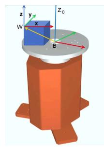
The origin of the workpiece in frame B is <sup>B</sup>p<sub>1</sub>
