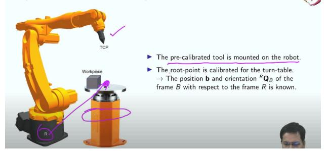
So, let us analyse that. So, the setup for that will be: the pre-calibrated tool is mounted on the robot, and the root point of the turntable is also calibrated. That means this point position, as well as orientation with respect to R, is now known. Now, I will mount the workpiece on top of this.
