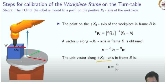
Now, the second step. So, the TCP of the robot is now moved to the point on the positive X0 axis of the workpiece. So, anywhere along the X axis, wherever you want to make it as the X axis of the workpiece, you touch it somewhere on that axis, and again, you calculate your next point, that is this one.
