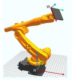
► The workpiece mounted (*flat surface*) on the robot's tool-flange needs to be calibrated so that the position and orientation at any point  ${}^{F}\mathbf{p}_{T} = [p_{x} \ p_{y} \ p_{z}]$  on the workpiece is known with reference to the robot's base frame.
