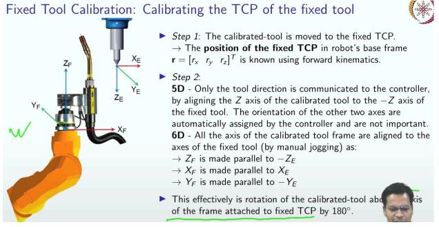
Now, let us begin with fixed tool calibration, that is, calibrating the TCP of the fixed tool. The tool is there in the workspace. You have to get to know the location of that tool as well as the orientation of that tool. So, that is our job now And what this robot is already having. It has a tool which is fitted at the end effector, That is, the tool flange of the robot.
