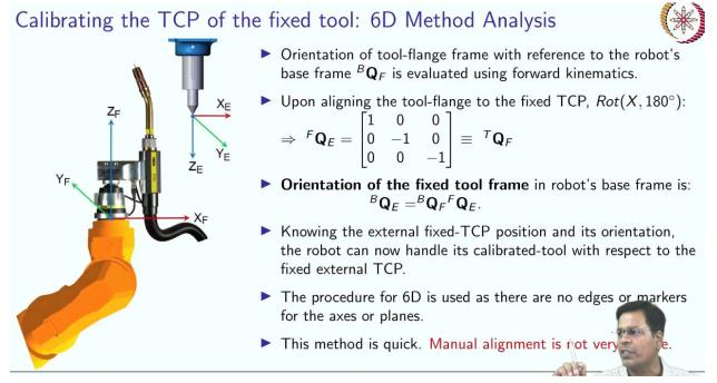
How? So, let us continue that. So, this is what we did, and orientation of tool flange: tool frame with reference to the robot base. This is evaluated using forward kinematics. So, this is quite easy and trivial now because, using forward kinematics, this frame, which is attached as the robot tool flange, you already know the orientation and position of this using forward kinematics, So you can quickly obtain. So, I now know this.
