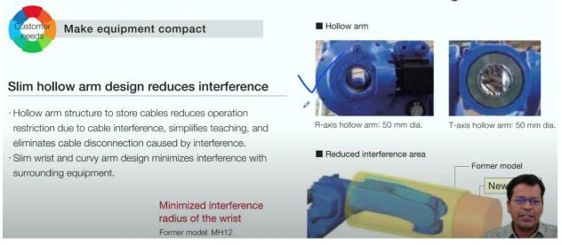
Once you see it specifying it is a hollow arm, it is a proprietary specification which is also given. Over here (blue tick mark), it has a hollow arm, which may be required for the arc-welding robots because you have to pass through many cables from between. And if it is so, if it is hollow, the cable does not interfere.
