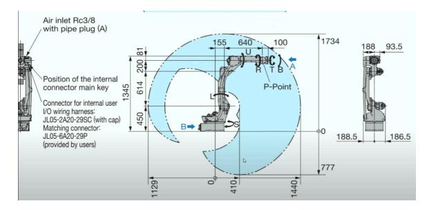
So, this is the workspace which is given in the datasheet. You see, it is the working envelope, this is the working envelope. So, this robot, this place, these are the places where it cannot go, and these are the places where it can go. You see, it is a complex shape all over, ok? It is a complex shape for the different views it is given.
