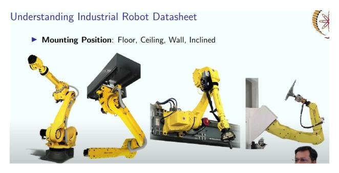
So, yes, one more very important parameter. Nowadays, at least on modern shop floors, you will find robots are not just mounted on the floor. In the video application, you also saw some of the robots mounted on the ground where it was picking huge objects and assembling the car body; one of them was hanging upside down, and it was picking the top portion of the car and putting it
