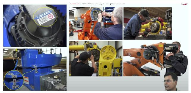
So, this picture shows typical maintenance which is carried out in the robot encoder and sometimes in the gearbox and some other. The whole of the motor is getting removed, you see. this kind of maintenance which are normally done if the robot has surpassed some definite amount of running hours, so planned maintenance also you do it sometimes after the breakdown.
