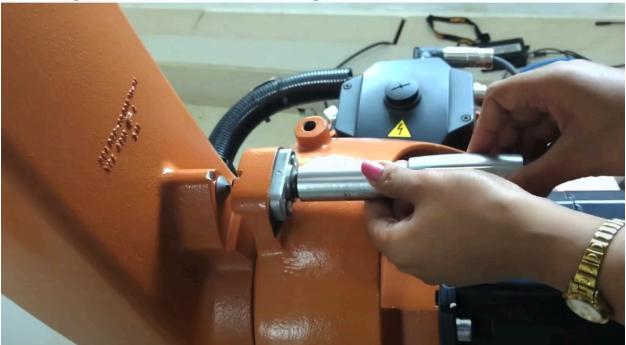
Mastering with an Electronic Measuring Device - KUKA Industrial Robot
