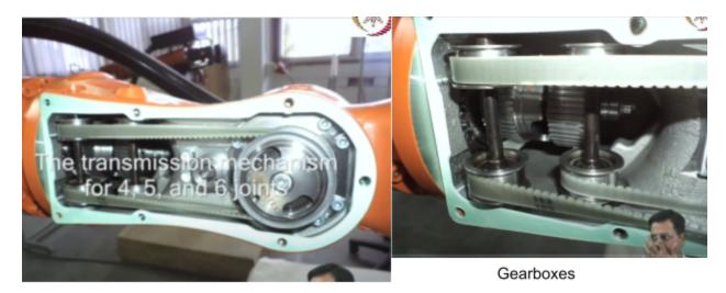
These are the transmission, which is there so that it moves. There are gearboxes which are inside. There are belts. There are pulley drives. So, it has started moving with the gearbox open now. So, axis 4 is moving. Now, you can understand. See, axis 4 is moving. Now, axis 5 is getting moved, and I have just put a marker so that you can understand the movement of the belt. It is a twisted belt. It is not a straight connected belt and that is driving the pulley.
