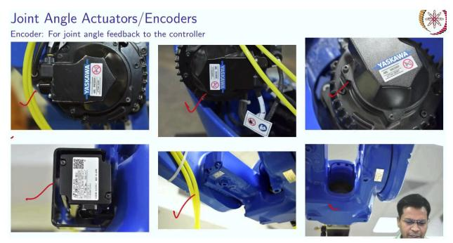
These are the actuators which are fitted with encoders at the end. These are not quite visible here,
