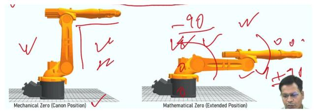
So, reference poses, or a variable which is there in the controller. What is that? It is an offset
