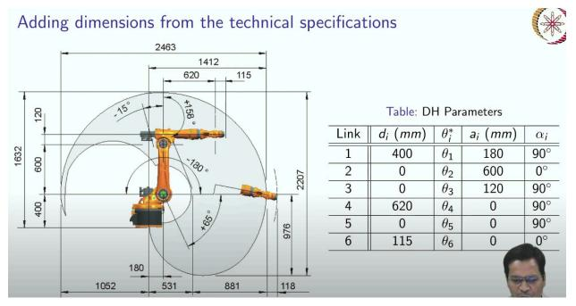
Now, let us populate this DH parameter table using the technical specifications which are given in the manual. So, you have just to put the distances as it is given in the datasheet. So, I'll just copy them from here. So, you see, it is 400 that is the offset. Offset from this point to this point. So, you see, it is 400. Now, theta 1 is the joint variable: 180, which is the distance between this
