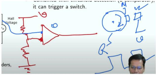
So, how to do it I will just explain here. If this voltage comes here, you have a comparator which is here that can give you output. So, there is a voltage level which is set here, using again like a potentiometer. We can set it. OK, so this is the voltage. This is the level with which I want to compare. So, here goes your input voltage so you can compare it with this. And so, as soon as it
