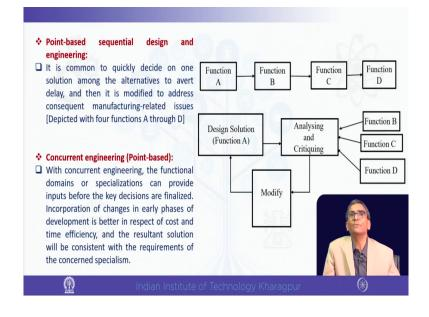
We will talk about that point based means say function A, B, C, D it is going sequential engineering, it is not concurrent ABCD sequentially. Concurrent engineering if it is point based say what happens, design function of a the lower one. The design function solution of function A which is being analyzed and critiquing.
