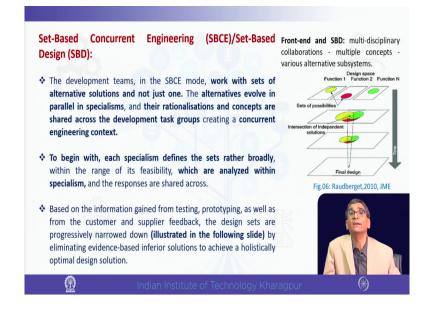
But in set based as you can see this figure you say Raudbergets figure which shows that the individual specialisms of different colors, they are having different sets. And through various layers they are being brought in closer together to see how the individual specialisms, the sets in individual specialism are matching and their intersection is giving us the design set.
