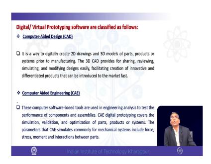
So, but briefly I have presented. So, that whenever you later on would like to revise you can just go to this slides and you will see it is a way of digitally create 2D drawings and 3D models of parts products and systems prior to manufacturing. The 3D CAD provides for sharing reviewing, simulating there are yeah of course, this some CAD apparent so called
