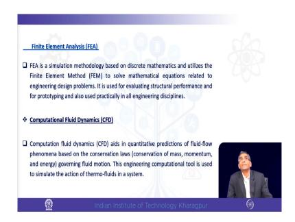
Finite element analysis you can study how the meshing etcetera is done if you intend to study it more, but this is an it is the principle. So, I at the moment I am not going to that there are so many lectures on a finite element analysis or finite element method. Finite element analysis is a simulation methodology which based on discrete mathematics and utilizes the finite element method, to solve mathematical equations related to engineering design problems.
