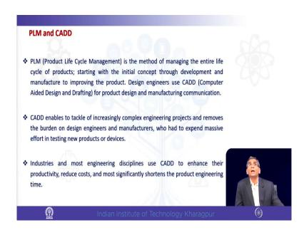
And we will talk about those. For example, PLM or Product Lifecycle Management is the method of managing the entire lifecycle of products. Starting with the initial concept development through the physical development or the design development and manufacturing. Manufacturing means this prototype and manufacturing to improve the product. So, that is the task. So, the CAD use of CAD is indispensable there.
