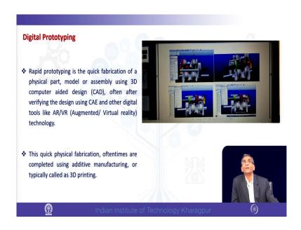
So, rapid prototyping as we said that it is a quick fabrication of physical part ultimately or assembly using a 3D computer-aided design CAD often after doing the performing the CAE that is Computer Aided Engineering or simulation is called. Like say when we want to test whether that component will be here will be able to bear the load or the or what is the force coming on that load component or what is the stress etcetera. So, those things we can test before actually we make it.
