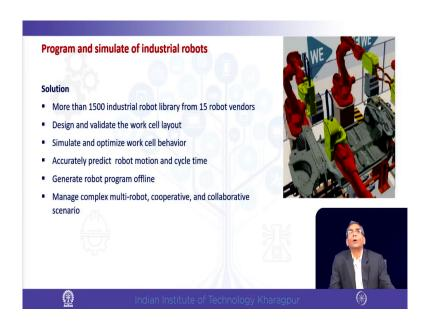
I have already said that it is a complex system. So, for example, a robot how robot would be simulated etcetera. There are say there is a library where one can call out of say 1500 industrial robot which are manufactured by say 15 robot developers or vendors, design and validate the work cell layout, simulate and optimize work cell behavior, accurately predict
