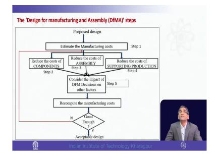
Here you see in one diagram we are bringing all the components. So, that you know the process the can be understood just in one page. A proposed design whatever is being conceived then that is a estimate the manufacturing cost that is step 1, step 2, 3 and 4 are parallel that is a component cost, assembly cost and support production cost.
