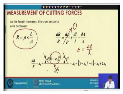
Therefore, if we have the resistance to be defined as  $\rho$  \* L/A, we can differentiate this and get this particular relation between the differentials. Where do we what is the origin of this one? This is simply resistance is equal to resistivity multiplied by length divided by cross sectional area. Resistivity for the time being we will consider to be constant, it is not affected by any of these physical phenomena which are occurring like stretching etcetera.
