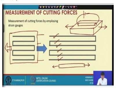
So, first of all if we want to measure strains, we can take the help of something called the strain gauge, how does the strain gauge work? The strain gauge it is like I will try to give you the idea in simple words. Suppose I have here a simple say a rod of whatever cross-section. So, this one I start pulling if I pull it, it will undergo a strain. Now in the same manner suppose I have a body, on top of which I have put a sort of conductor it is absolutely cemented onto the body.
