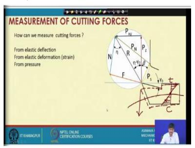
How can we measure cutting forces? Cutting forces can be measured from elastic deflection, now what do we mean by that? We mean that you know just a moment if under the action of cutting forces this tool deflects; why should it deflect? Because the force is in the other direction, this force mind you is on the chip, the cutting tool experiences this force because of which this is the force on the cutting tool.
