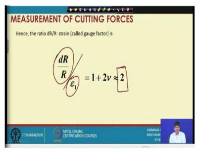
Just a moment, dividing the equation throughout by  $\varepsilon_1$  we get dR/R by strain, that means change in resistance per unit strain is equal to 1 + twice Poisson's ratio. Because we will get  $\varepsilon_2$  by  $\varepsilon_1$  here, and that can be assumed to be equal to 2, which means that change in resistance per unit resistance divided by strain is actually a constant, these 2 things are proportional.
