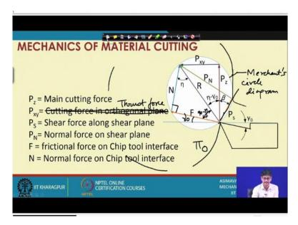
So, having agreed about that let us come to the different relationships which now exist for the resultant forces on the cutting tool. What do we mean by the resultant forces on the cutting tool? On the cutting tool the forces which are being applied by the chip they are normal force and frictional force. I mean we can break them up into such components; there is a single resultant force what we know about that force is that it is on the orthogonal plane.
