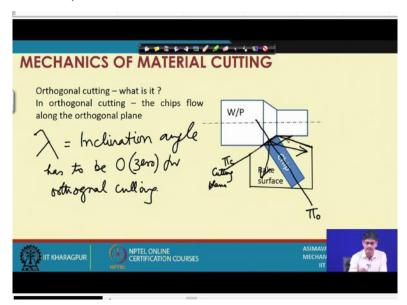
So, here first of all we see a chip coming out of the cutting zone in a particular direction and you will notice that roughly I have indicated that the chip is coming out in the orthogonal direction. What is orthogonal direction? This one is the trace of the cutting plane seen from top, cutting plane or  $\pi_c$ . This one perpendicular to it and perpendicular to the reference plane must be orthogonal plane.
