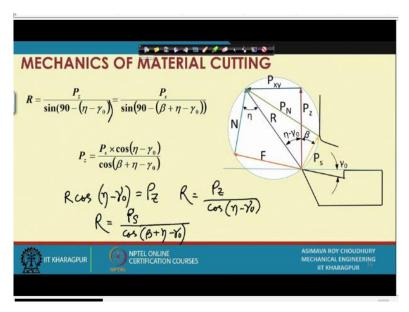
First of all we can establish a relationship between the resultant and some of these components in this manner. We can say the resultant force multiplied by  $\cos{(\eta - \gamma_0)}$  is equal to  $P_z$ . So, how do we establish that, let us see this is  $\eta - \gamma_0$  and we are writing I think we can do it in an easier manner than what is written. First of all let us see what we have stated here.
