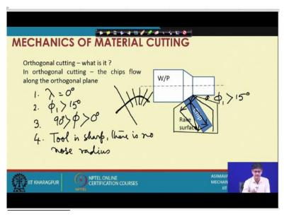
So, the auxiliary cutting edge also does some cutting and if the chips emanating due to that cutting effect they will have a chip velocity in this direction while the component of velocity from the main cutting edge might be higher than that but they will combinedly define a particular direction of resultant chip flow. Therefore, this is another possibility of deviation of the chip from the orthogonal plane.
