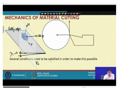
So, next when the chip is coming down the orthogonal plane and when there is no angle on this side this is orthogonal rake angle, if this is 0. So, that means sideways there is no tilt, in that case the pull forces of this body coming down the inclined plane is only defined by the normal reaction and the frictional force.
