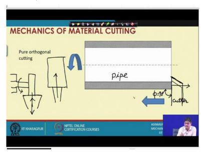
We sometimes refer to some cases as pure orthogonal cutting. What is pure orthogonal cutting? If we completely remove the auxiliary cutting effect I mean the cutting contribution of the auxiliary cutting edge if it is completely removed from the picture in that case and also the other effects which are taking place, if they are completely removed in that case we can have a situation in which purely orthogonal cutting is taking place with absolutely no interference from other factors.
