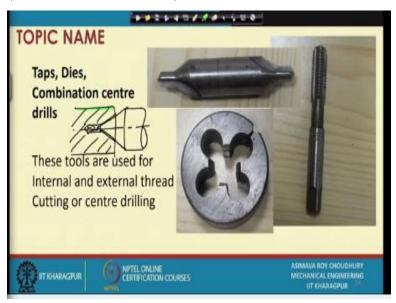
This is called a combination centre drill; it makes such a hole in material. If you have a material like this combination centre drill will typically produce a hole of this type, what is the use of such a hole? Such a hole allows us to put centre inside this, which holds it properly, locates the axis of this hole aligned with this particular centre. I mean the axis of this centre and the axis of the body which is being held, they will become aligned together.
