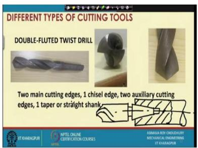
This is a drill tool, what are the characteristic features? A drill what you call it? The drill which is shown is a specific type of drill, what is it called? It is a double fluted twist drill, there are 2 cutting lips here, main 2 cutting lip, there is an auxiliary; there is a chisel edge also. This is one such in this one this is the main body, and this is the shank, the shank portion goes inside tapered hole in the spindle which is generally rotating.
