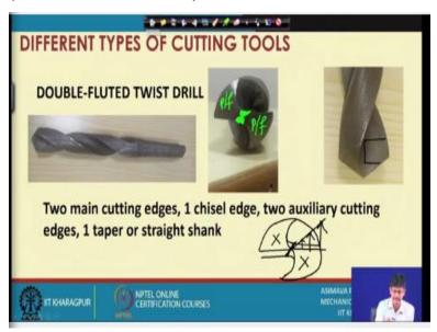
Yes, just a moment, this is the chisel edge let me underscore it in order to emphasize its importance. This is the chisel edge, what does it do? So, here there is the chisel edge, it cannot be seen from this side, it is a chisel edge. What does it do? What is its role? As we have to provide a body to the drill, ideally we would have liked this particular configuration let me show you. Yes, we would have liked this configuration, this is visible.
