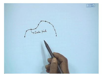
Suppose there is a designer who has designed a very nice looking car body and he asks the asks the ask the person who is handling the geometrical aspects of the design, pass a curve through these points, so these are now not the control points through which the curve has to essentially pass and therefore, after successfully drawing of the curve, the Bezier curve could
