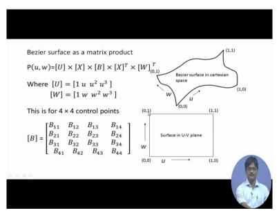
So if we similarly we look at the equation of the sorry formula of the Bezier surface, it looks this way. The Bezier surface has this U parameter varying from 0 along the edge up till this point where it takes up the value of 1. Here also allow all these lines moving from this side to
