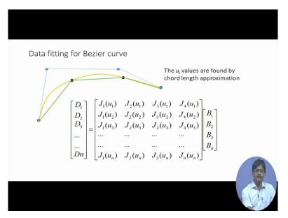
So we will have grid lines X parallel to Y parallel to X appearing here, which will be the isoparametric lines. Coming to data fitting, what we mean by data fitting? Data fitting means that control points may be controlling the surface but designers might be interested to have a curve, which initially passes through a number of points. Let us have a look at at this particular case.
