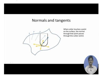
So this is the cutter, when the cutter is touching the surface at this point the normal to the surface will essentially contain the centre of the cutter okay. So the normal to the surface will essentially contain the centre of this spherical end of the cutter, so we understand that this normal which is emanating out at this point of the surface it is passing through this centre which is shown, so we make use of this... This figure will make it clear.
