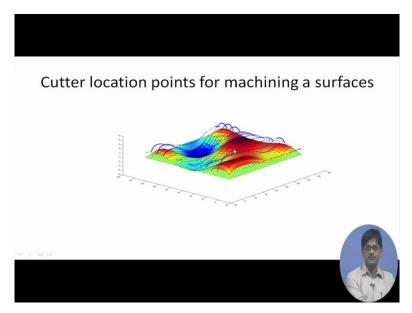
Here we have shown a surface and you can see some small red or rather blue dotted lines just over that particular surface, these are cutter paths that mean the centre point of a ball ended cutter path with these locus point as the centre points of the ball end okay, we will have an example later also in order to understand this.
