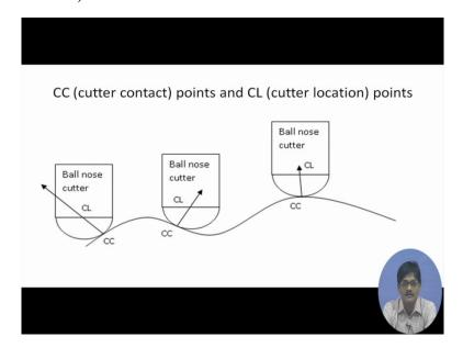
First of all, we are differentiating between 2 types of points in connection with 3 axis machining that is, if we have a ball ended milling cutter in connection with the surface, the point at which it touches to the surface, it is called cutter contact point CC point. So there are three contact points, clearly cutter contact points are not one steady constant point with
