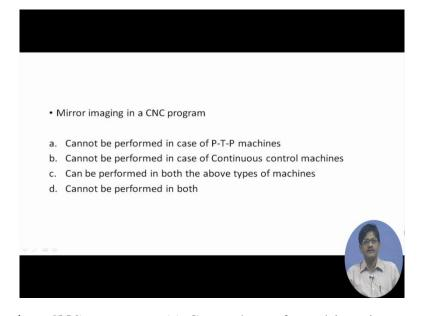
Mirror imaging in a CNC program... (a) Cannot be performed in point-to-point machines, (b)cannot be performed in case of continuous control machines, (c) can be performed in both the above types of machines, (d) cannot be performed in both. So D is obviously wrong, if it cannot be performed in both it would not have existed. And A and B they are also wrong, Mirror imaging can be carried out both in point-to-point as well as continues control machines, so option C is correct.
