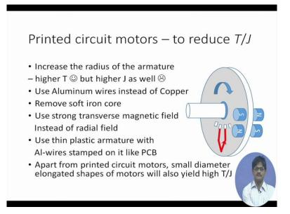
What is the basic idea in this Printed circuit motors? It is 1<sup>st</sup> of all accepted that increase of radius of the armature will bring in higher T because torque is proportional to the 1<sup>st</sup> power of radius, but unfortunately it will bring a higher value of J that means the denominator will also become higher so that ultimately this term will become very low because it is proportional to
