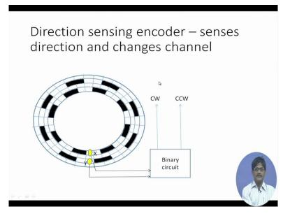
So, let's have a quick look at the direction sensing encoder. We have 2 rows of holes and they have a stagger that means there is a difference in phase so that, these black portions are the transparent places and these white portions are opaque, so that if we have 2 light emitting devices with receptors on the other side, we will have pulses coming out with a phase difference from these two. So if you notice, we have written here X and Y, so if this encoder
