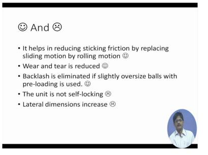
And it has some other advantages and some disadvantages also. If we use a recirculating ball screw nut mechanism, it helps in reducing sticking friction by replacing sliding friction by
