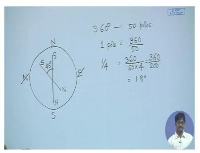
Let us have a quick look at simple model of 4 steps. This is my magnetic needle, this is south pole, this is north pole and this one the stator is going to have say at one point north and
