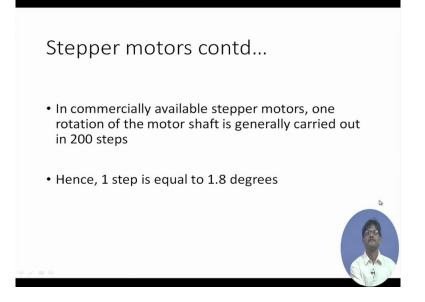
So we generally have stepper motor available which can carry out 1 complete rotation in 200 equal angular steps therefore, one step is = 360 degrees divided by 200 = 1.8 degree, this is generally the standard angular step available with commercially available stepper motor. Other options are definitely there, but we will be generally dealing with this particular value.
