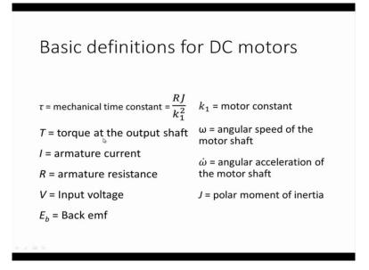
These are the definitions like this T is torque, I is the armature current, R is the armature resistance, V is the input voltage to the two motor and the motor develops back EMF due to electromagnetic induction, etc, all these things we will be able to understand while we are going through the analysis.
