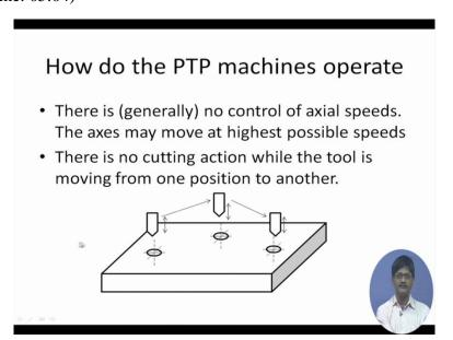
So this is a typical picture giving at definite locations some operations are being done. So this is a drill like cutting tool, it is supposed to move down, carry out drilling operation, come up,
