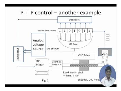
So in this figure we see the depiction of another type of point-to-point control, let us see 1<sup>st</sup> of all what is the prime mover. The prime mover is a DC motor, this DC motor connected with a gearbox as previously is also connected to a lead screw okay. This lead screw nut combination produces linear motion of the table.
