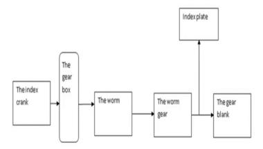
So, what do we have now? To start with, this one is what we have at present. This one is what we decided that this gearbox is not going to serve the 2 purpose of rotating the index plate properly and the index gear blank properly at the same time because they have different requirements of the value of the gearbox ratio if it is placed here.
