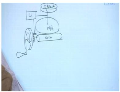
If you allow me to draw the figure, it looks like this. This was the index plate, through this past the crank. This crank went to the worm; this worm was connected to the worm gear. Worm gear had on one side your job. On the other side, it had a gearbox U which ultimately gave its power through bevel gears to this plate. This was what we had index crank, worm, worm gear, gear blank, gearbox and this gearbox was controlling the power to an index plate which was now rotating.
