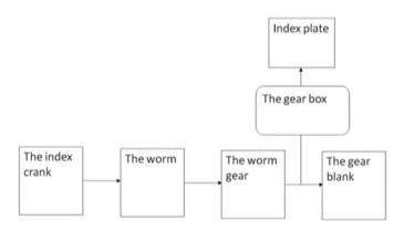
Now, let us quickly discuss the positions of the gearbox in case of milling. Now, that we have become conversant about the positions of the gearboxes in different cases of hobbing and shaping. What do we exactly mean by this? We mean that in hobbing and shaping we had come across different laws or rules with the help of which we were establishing the uniqueness of the positions or locations of the gearboxes in the kinematic structure.
