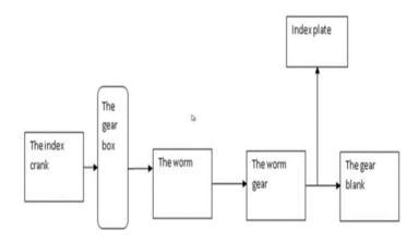
Why not this? So, from the logic that you had learnt about while locating different gearboxes at different places, I would like you to judge, whether the gearbox can be placed just after the index crank. Just after the index crank, you place it just after the index crank so that the worm gets a different rotation, from what it was supposed to get. And the worm gear gets some rotation etc. What problem would it give rise to? So, let us have a discussion on that.
