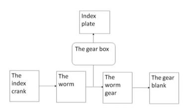
Let us take yet another possible location of the gearbox. What about putting the gearbox here? Ahead of the worm gear after the worm so, if it is after the worm, therefore, worm gets the required amount of rotation and if we do the calculation now. It will be, index crank rotation multiplied by the worm rotation, these 2 are going to be the same and after that, if we have a gearbox that is going to give us the index plate rotation. So, let us write down index crank rotation.
