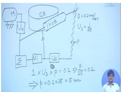
So, let us quickly draw this particular figure. This is the hob. This is the job and the speed is obtained by the position of the  $U_v$  here. This is the motor, hob, gear blank. So, tap the power from here, this is our differential. This must be  $U_i$ , this is the connection to the work piece and this is our  $U_s$ .  $U_s$  feeds vertical screw with the help of which the hob comes down.
