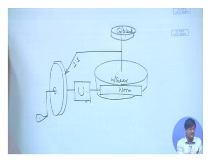
This is our index crank. This is our index plate. This is passing. We are now proposing gearbox here and worm here. Worm gear in contact with the worm. And this is our gear blank and we simply tap this power and 1:1 we give this particular connection. Why not place it here? Are we going to face any problem? Or just because we have studied it in different books it should be placed here.
