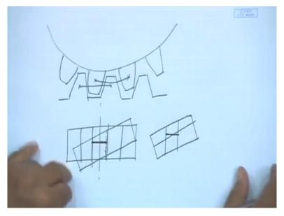
We have this sort of a relation existing; say this is the basic gear. And with this one we are drawing, these being the gear teeth, we have the hob which is actually a worm with cutting edges. This sort of a relation is existing, which means the circular pitch is equal to the linear pitch, but if you remember, in the other view, the worm gear being like this is being a spur gear, the teeth are of this type and the hob has to be at an angle.
