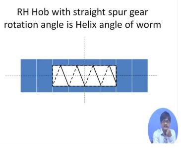
Second case, let us try it out. The blue one is the gear to be cut. And these white vertical lines, they are the traces of the teeth. Now, let us give it a rotation and see what happens. Yes, this seems to be it. Therefore, the dotted lines are matching with the direction of the teeth being cut. And therefore, we say that for cutting a spur gear with right hand hob, the rotation angle is simply the helix angle of the worm.
