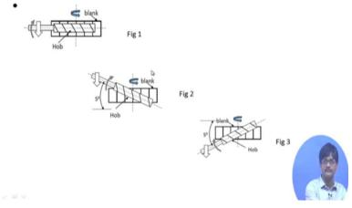
I hope you can read it. The helix angle of a hop cutter a right handed helix is 5 degrees. It is used for cutting straight tooth spur gear. Axis of the hob cutter should be? As in figure 1, as in figure 2 and as in figure 3. Which one is correct or none of these? So, let us look at these. This one the axis of the hob is crossed with the axis of the blank that means at 90 degrees. But this will not do because the thread of the hob has to align itself in the direction of the teeth being cut.
