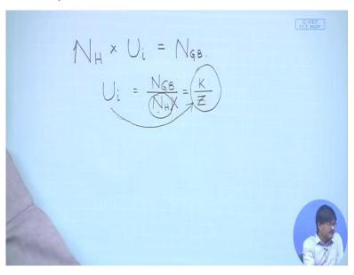
We know that starting from the hob rotation, suppose how much, rotation of hob  $(N_H) \times U_i$  must be equal to, we are considering that there are no other machine elements in between no gears, no belts, no bevel, no worm, worm gear etc.
