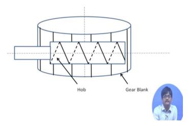
Now coming to this. This problem also we had identified. How do we decide, whether a particular hob is correctly aligned with the work piece or gear blank? For that let us see we are taking the case of a spur gear with straight teeth and this is a right handed helix. So, the dotted one is the one which is touching, on the side of the gear teeth in contact with the gear teeth.
