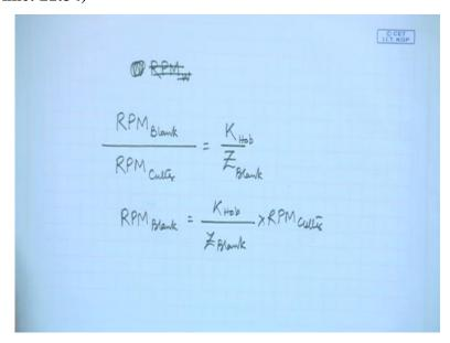
Since, let us, write this down RPM work piece, or we have used the term blank. So, let me cut this:
