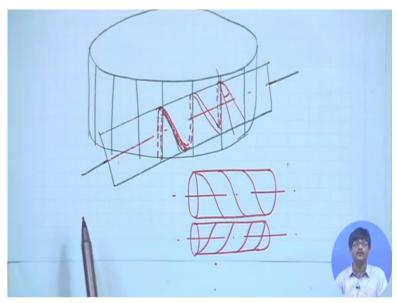
This figure will explain a number of things which we have discussed up till now. If we are cutting straight spur gear teeth and a particular hob cutter is in contact with it, say this is the hob cutter. First thing that we should notice is that the hob cutter is inclined. When we are having ordinary worm and worm gear mechanism pairs the worm is not inclined. Why? Because the worm gear teeth they are slightly inclined they are inclined at the helix angle.
