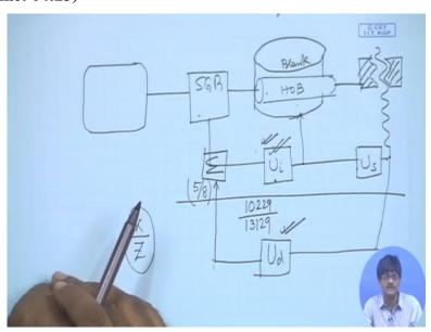
Instead of that, we have this particular problem that cut a spur gear of the same number of teeth with a particular helix angle. We can redefine  $U_i$ , so that instead of having the ratio  $\frac{K}{Z}$ . It will have a slightly changed value of this particular ratio. So, you can have that but the simple problem is, if you have of such a particular relation you will find that  $U_i$  comes out to be very very difficult to get.
