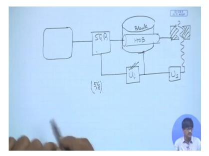
For that, let us have a quick look at the setup. What does the setup consist of? Once again there is the motor, we have the speed gearbox and from there we are having hob rotation. From there, we are having differential, suppose I intend not to use the differential. In that case, what should be my setup? I should have  $U_i$  here. I should rotate the, let us try it this way. That is it.
