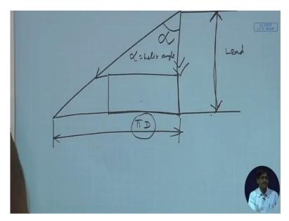
Let us have a look at it on the figure. This is our work piece and therefore, if we unfold the full work piece this comes out to be  $\pi D$  circumference. Now, that the helix should be such that, this is equal to lead of the helix and this we know as  $\propto$ . The helix angle and therefore, helix angle is  $\tan^{-1}\frac{\pi D}{L}$ . So,  $\propto$  equal to helix angle, so, we have to find out how much is this motion downwards?
