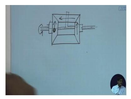
So, this will remain in position and rotate, because let us draw a figure. This is the figure. I have 1 here at this place. So, I am rotating this one this way. I am rotating this one this way and therefore this gear will be rotating this way. If these are equal in magnitude, it will simply remain in position and rotate. But suppose I had rotated this one in this direction. What would have happened? Same rotation both of them in the same direction.
