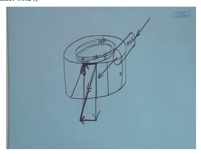
First of all, on this particular figure. If I have a blank on which if I have matched the rotational ratio of the hob with the workpiece, if this rotational ratio is matched, when say the meridional plane x comes under the hob, it gives a cut. So, this way each and every, say let us call these
