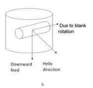
This is the velocity relation which we have already discussed. That means, the hob has downward motion and the blank will be given extra rotation because of which they will be tangential motion, the resultant of both the velocities will give rise to the helix direction.
