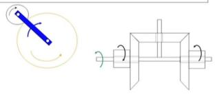
An example of differential with bevel gears.
