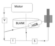
And if you look at this, this was the accepted position. And this was the change position and we noticed that the location of I in this particular position unfortunately is going to change the hob RPM and that would result in a different cutting speed. And that is going against our basic resolution that one gearbox should affect only what it is intended to and nothing else. Change in speed should be controlled by the change in U<sub>v</sub>, change in speed.
