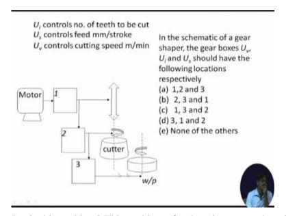
Next problem: what is this problem? This problem after learning so much and discussing so much about fellow gear shaper; it should be extremely simple for you. First of all, we have stated that  $U_i$  controls the number of teeth to be cut.  $U_s$  controls feed in millimetres per stroke.  $U_v$  controls the cutting speed in metres per minute. I have just jumbled it up.
