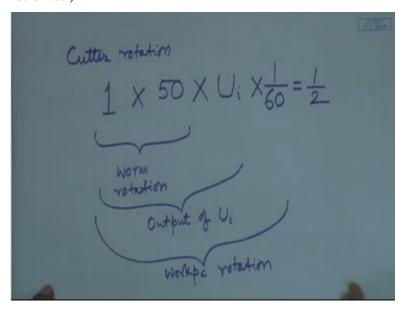
First of all, we put the cutter rotation to be 1. Since it is the same as the worm rotation, then we multiplied by  $\frac{50}{1}$ , the reverse ratio to get the worm rotation. After that through the bevel gear pair, we come to the main line. It is just like a car backing off from a by-lane on to the main road.
