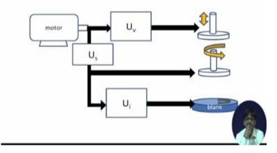
What about this?  $U_v$  is here;  $U_s$  is here;  $U_i$  is here. Let us take them one by one. Since, in fact, we can move very fast through it now. We can say here if  $U_v$  is connected to the motor and  $U_s$  is also connected to the motor directly, something is going to go wrong. What exactly? Suppose you change  $U_v$  now, number of strokes get say doubled, but  $U_s$  is not affected because it is drawing power from the motor directly.
