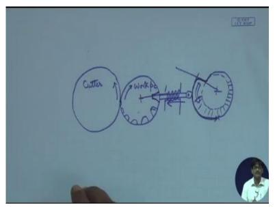
Infeed takes place this way. We have the cutter. We have the work piece. Initially, they are touching tip to tip. There is no cutting taking place and then they start, when they are rolling at the same time, this is moving in. Gradually, these teeth will be getting higher and higher values of cut. That means when this one comes here, it undergoes this amount of cut.
