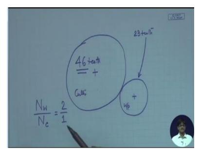
We have this as the cutter. The cutter is also a gear as you noticed in the simulation and say, this is the work piece. Now, how are we going to decide how many teeth are going to be cut? Suppose, I decide that I want to cut say 23 teeth. If I want to cut 23 teeth on the work piece, suppose, the cutter is having 46 teeth, then first by calculation, I have to find out the correct outer diameter.
