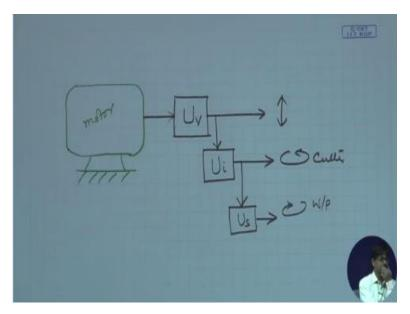
This is our motor. This is output from the motor. We have gearboxes, up down movement, rotation of cutters and rotation of work piece. And here, we put  $U_i$  and here, we put  $U_s$ . And here, we are having  $U_v$ . That means if I change the positions of  $U_s$  and  $U_i$ , what is going to happen? So, first of all,  $U_v$  serving its purpose. And after that,  $U_i$  is outside the loop of the cutter and the work piece.
