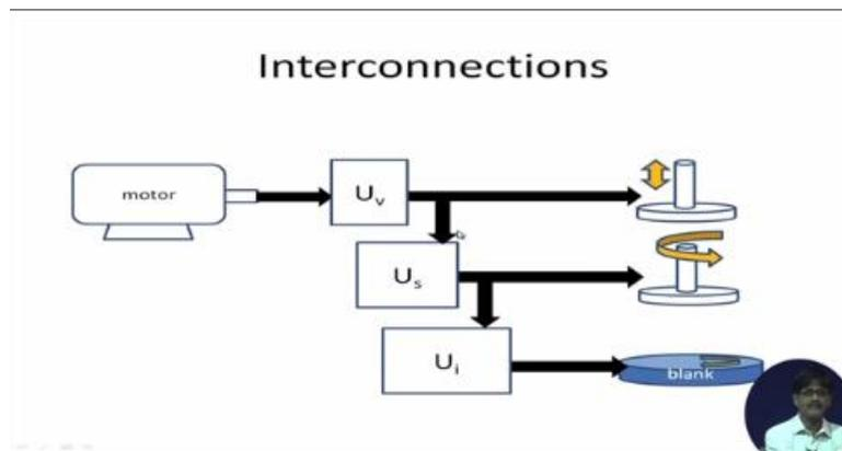
So, let us have a look at this particular interconnection. What do we notice here? The motor is first of all serving  $U_v$ , the speed gearbox. So, it means that the power is flowing from the motor to the speed gearbox. How does the power flow? So, the motor shaft is rotating and that shaft goes inside the gearbox  $U_v$  there.
