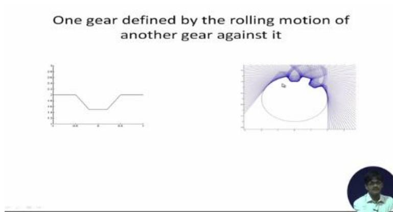
This shows that this is the rack geometry that I have and I am rolling it against. I am moving it as if it is rolling against a virtual gear and the continuous positions of the rack, they are recorded here. And when I am taking the conjugate envelop, this one, conjugate means just the opposite space. So, all these other positions of the rack and when I am taking the conjugate space, I find that it is generating gear tooth shape.
