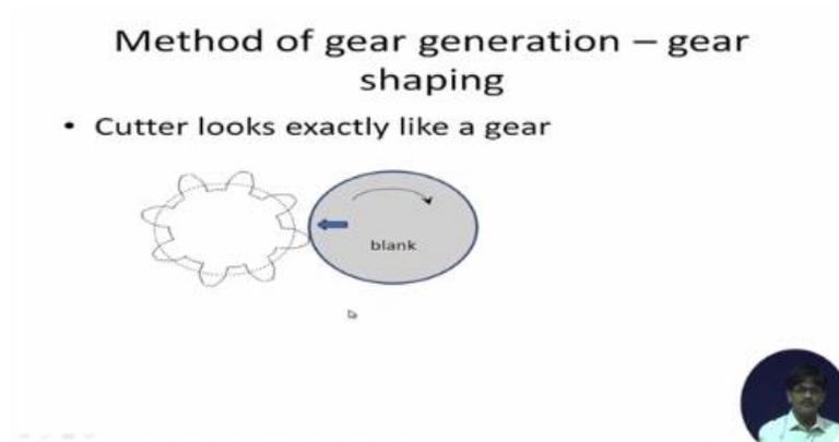
So, let us have a look how the method proceeds in case of gear shaping. This is the cutting element. It is made of absolutely hard rigid material which is not deforming and in contact with it we have the gear blank that is also metallic or it can be plastic or some other material, but it is relatively softer and this one, because conventional cutting is going on so work piece material has to be softer, but it has to be cut.
