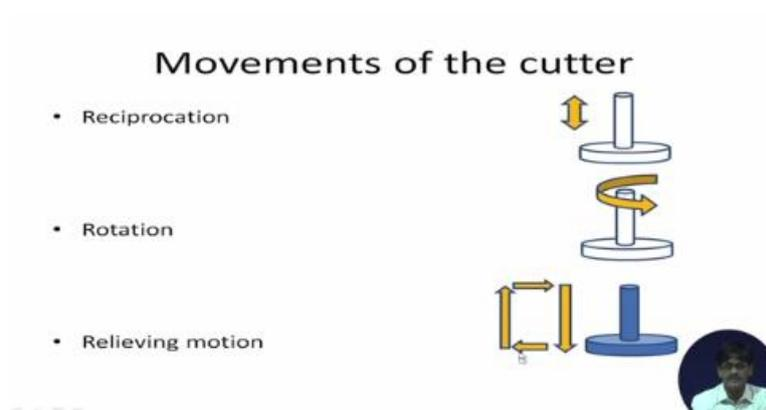
So, what are the movements that we are providing? We are providing as we have seen reciprocation. This reciprocation provides the cutting action. The cutter cuts off all the material it finds on its way and that way, material is removed by cutting action. No pressing, no damaging, no denting, but cutting. In addition to that as we have noticed, the cutter also has a rotation because we have to create a situation in which as if cutter and the work-piece, they are already formed gears.
