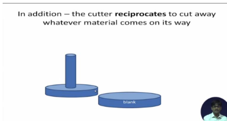
This is the cutter. This is the blank as the cutter is also moving this way together with rotation of the cutters, rotation of the blank as we have seen before and movement of the blank towards the cutter. So, this reciprocation removes all the material the cutter meets on its way. Remember the cutter is having teeth on its periphery and those teeth have sharp edges and they are given cutting angles in order to facilitate material removal.
