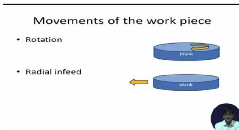
Work piece is also rotating because we are creating a condition of rotation of the cutter and the blank together. So, this motion has to be provided as well and work piece is having radial infeed which we have noticed during the simulation. Why does the work piece have gradual towards the cutter radially it is moving? This is because the cutting action is made to increase slowly from 0 depth of cut to the full depth of cut.
