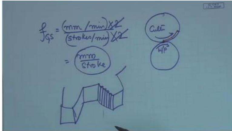
If you kindly have a look here, it is something like this. So, the feed in case of gear shaper, millimetres per minute by strokes per minute, strokes per minute is getting doubled; millimetres per minute circumferential movement, it is like this.
