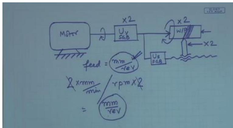
And I think that will make subsequent discussions extremely clear. On the lead, we have a motor from which we are drawing power and if you remember, we have the location of speed gearbox. Let us call it SGB, speed gearbox here and after this, just like as in the gear shaper, we have the spindle to contain the work piece and withdraw the power from here for  $U_s$  feed gearbox and from here, you might be having a lead screw.
