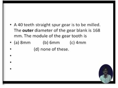
A 40 teeth straight spur gear is to be milled. The outer diameter is 168 millimeters; the module of the gear tooth is, so how do we solve this question? We say that the outer diameter of the gear blank in case of straight spur gear is equal to we will write it down here.
