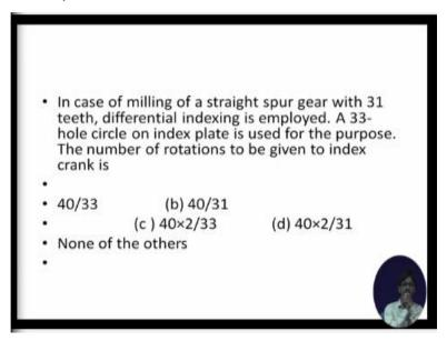
In case of milling of a straight spur gear with 31, teeth differential indexing is employed. A 33 hole circle on index plate is used for the purpose. The number of rotations to be given to index crank is? So, this is now very simple for you people because you have already done 2 problems. So, what is asked for?
