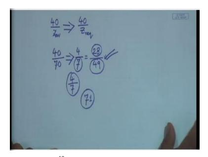
As we know the magic number is  $\frac{40}{Z}$  and in differential indexing what happens? The  $Z_{required}$  is not there, so move by  $\frac{40}{Z_{available}}$  and the machine will adjust through the mechanisms that change gear and all those things. This will be converted to  $\frac{40}{Z_{available}}$ , gets converted to  $\frac{40}{Z_{required}}$ , that is a function of that gearbox and all those things. So, in this case how much do we have to rotate the crank?
