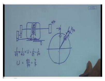
For that please have a look at the paper, what we generally do? Just to remind you is this, that we have this dividing head. On the dividing head we have this particular index crank sticking out, this is the index plate. And this gets connected to the worm; this one to the worm gear, worm gear feeds the workpiece, that is your blank. On this side we have those gears etc. This one connects up through a bevel gear to the index plate.
