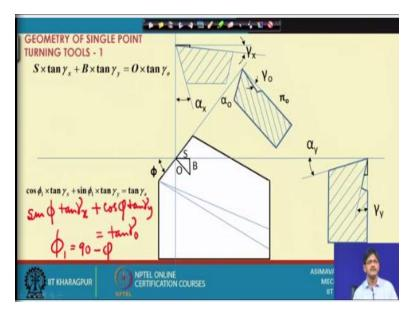
This is the first exercise that we have in angle conversion. For example, suppose I am interested to know what is the relation between orthogonal rake here and the 2 rake angles in the American system  $\gamma_x$  and  $\gamma_y$ . So, I start from here from this relation, what does this relation state? It states that from this point if we move down the rake surface in the orthogonal direction we will reach a point.
