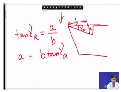
A tool in any section if I am going down by this distance vertically, say I name this a, if this angle is given say  $\gamma_a$ . Sorry if this distance is not given a is this and say b is this much,  $\gamma_a$  is this. Therefore, in this case I can write  $tan \ \gamma_a$  is equal to simply a/b, perpendicular by base. This means that I can express 'a' as  $b*tan \ \gamma_a$ , this is the relation that we will be using extensively in our calculations.
