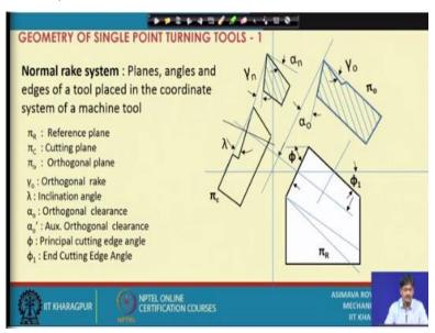
So, it would look somewhat like this, we have this tool in the plan view, we have the section in the orthogonal plane, we have the view in the cutting plane. And then if we make a section this way sorry I have not shown the section arrows, if we make a section along this particular line then we will get a sectional view in which normal rake will be coming out here.
