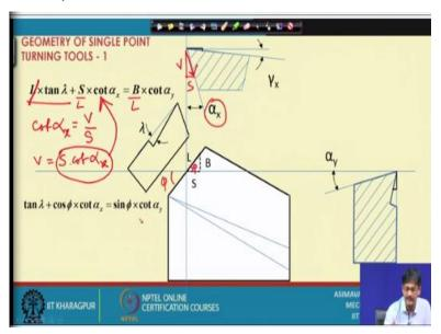
Next, so first let me, now we come on to something different, up till now we have established relationships between orthogonal rake angles now we will be establishing relationships between clearance angles. And since the inclination angle is shared between the rake surface and the principal flank, we can have a relation existing between the inclination angle and the 2 principal clearance angles in the American system.
