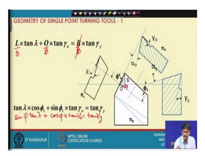
So, here we have another relation in which we are bringing in something else. That is a relationship between back rake and inclination angle and orthogonal rake. Previously we were working with back rake and side rake and one of the angles in the orthogonal rake system. Now two of the angles of the orthogonal rake system can be brought in and only one angle of the American system can be considered.
