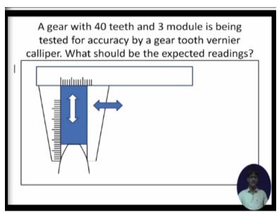
So, I will take this opportunity to introduce one gear measuring method I mean testing of gear teeth whether it is made well or not by discussing about the gear tooth vernier caliper. We had slightly referred to this in our previous lectures but not solved any particular numerical problem,
