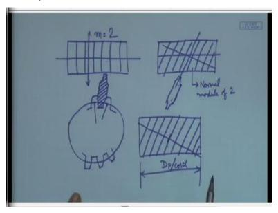
If you have a look here, in case of spur gears this is the direction in which their teeth align and on the other view if you look at this, the teeth are this way. So, this is basically the cutter, the cutter is physically defined piece. And therefore, it gets defined by this particular gap and as we have studied previously this gap is equal to this particular distance not the angle. This particular distance
