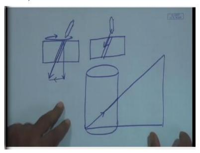
If you have a look once again, once we have understood that even though this is the job the cut is going to take place this way. So, the cutter which is once again that same cutter that we have used for spur gear milling, that same cutter has to pass this way now. We have ensured the motion to be in this direction by the combination of rotational motion and straight-line motion.
