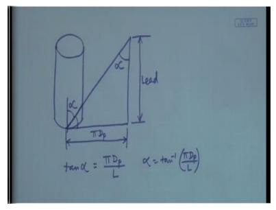
This is your cylinder, this is your helix and you unfold it, so that you get a triangle, what is this triangle having? It is having this side equal to  $\pi D_p$  that means the circumference of the pitch circle. It rides up by the lead in one rotation, so this must be equal to lead. And what is the helix angle?
