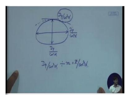
This is what it looks like now, this one is twice be  $=\frac{D_p}{\cos x}$ , this one if you consult the figure, you will find it will be equal to  $\frac{D_p}{\cos^2 x}$ . And we have to find out at this point what is the curvature, what is the radius of curvature of the gear? That radius of curvature will have a corresponding diameter. Radius of curvature double of that diameter of curvature, that diameter will be able to accommodate a certain number of teeth.
