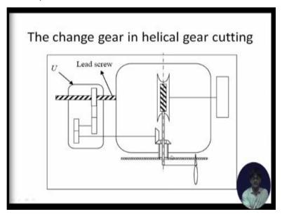
So, now for the calculations, now those who had problems in understanding what we mean by locking of the index plate with the index crank, here is a quick view at that. This is our job, this is our worm and worm gear and this is our index plate and this is our index crank. Right from the lead screw if you follow up, lead screw, gearbox connected with the index plate through these 2 bevel gears and you climb up to the index plate.
