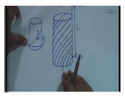
If we have a particular cylinder and on that by some means if we are tracing a line. This line will be executing a helix, I mean the tracer will be executing a helical line if you have circular motion of this disk combined with straight line motion of this pencil. If they are proportionally moving, that means if this is moving a certain number of units, this moves by a proportional number of units and this proportionality is maintained.
