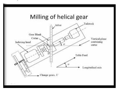
So, we have finished most of the discussion on differential indexing, so, let us start with helical gear cutting on the milling machine. What do we have here? We are seeing the milling machine from the top, the milling machine table, you have already seen this one in the previous lecture and let me quickly identify the various parts which are present here. For example, this is the gear blank, it is basically a disk that means cylinder shaped job with a short height.
