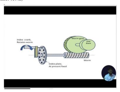
First I take out this pin from the index plate and rotate this by 20 holes on a 30 hole circle and put the pin down that means I am sealing this particular initial rotation 20 holes out of a 30 hole circle; put the pin down and after that if I still rotate the index plate is going to rotate with
