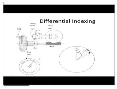
So, indexing with feedback is called differential indexing. And let us have a quick look at it. What does this figure show us? This figure shows us once again, so let us go through things that we already know this is our index crank, this is the worm axis, this is our worm gear, this is a pair of bevel gears which turn the rotation by 90 degrees. And we find that there are some gears now existing which rotate the index plate. In simple indexing we had not rotated the index plate.
