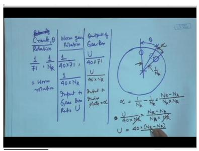
We do the calculation this way. The crank how much does it rotate? First hole, second hole, virtual hole, this is the crank rotation  $\theta$ , how much is it? This must be equal to 1 by the number of teeth we cut, this is the virtual hole position and this must be equal to  $\frac{1}{71}$  in our case.
