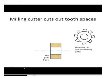
So, this is the cutter, it rotates about this axis, the axis is vertical to the plane of a paper or the screen, so that is why it is called rotary disc type, obviously it is shaped like a disc its width perpendicular to the plane of the screen is much smaller, form milling cutter in the next view we will see the form that it has it is the conjugate, as we said, of the tooth space to be cut off or removed from the gear blank.
