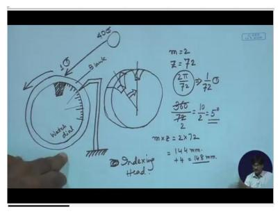
If you look at this particular gear, if I have to remove this material in order to create teeth, in that case after this has been cut I have to give it a rotation of this much and here I have to give a rotation up till this point, how do I give that? So, let us do some calculations to find out how
