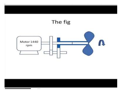
So, we discussed a possible configuration in which the motor is rotating here and there are 2 gears which are increasing the RPM in this ugly shaft, these 2 gears are sharing the RPM and this is finally giving it to another gear which is loosely fitted on this shaft and connected to the fan, so that ultimately the fan rotates at the required RPM. What sort of increase is there? So, if you divide the RPM.
