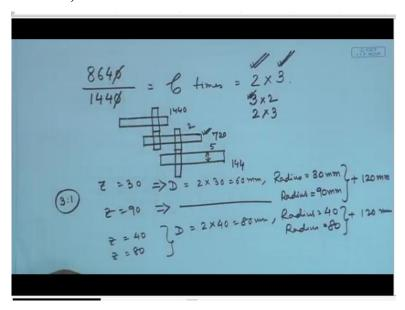
Let us work it out on the piece of paper  $\frac{8640 \text{ rpm}}{1440 \text{ rpm}}$ , if you calculate you will find 6 times increase of RPM is required and as shown in the figure it has been provided that we should try to achieve it in 2 steps. Now this is 2 x 3, so let us have a multiplication of the RPM 2 times and then the multiplication in 3 times but we first do 3 and then 2 or then 2 and then 3, or does it really matter if I am doing 2 first and 3 next etc.
