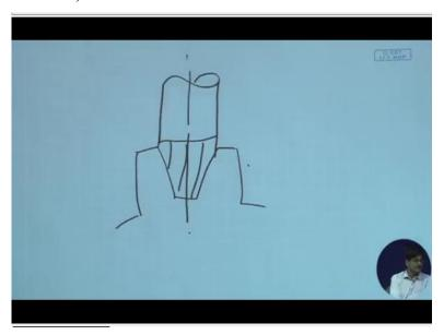
Have a look please, this is the end milling cutter, it rotates this way and removes material, it is not as popular as the other configuration of rotary disc type form milling cutter.
