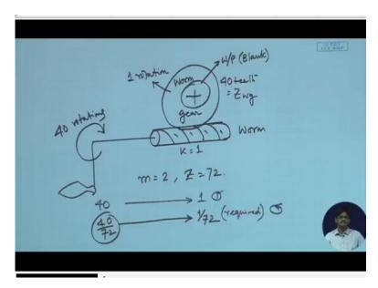
The indexing head basically consists of, this is the main working part of it, this is a worm, now you are quite conversant with the worm and the worm gear can be here up, can be here to the side etc., let us draw it up, it has a worm gear connected to it. What is worm gear doing? This one has say 40 teeth and this one is say k = 1. So, if I give 40 rotations here, this is going to give me one rotation only.
