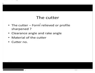
Now so we have discussed almost everything about the cutter, as we discussed it is a form milling cutter, so it is it falls under the category of form relieved cutters where the sharpening is done on the rake surface, never on the clearance surface because the clearing surface is having a definite form it cannot be disturbed and only the material cutter has not been discussed, it can be made of high speed steel, it can be made of carbides etc. Cutter number we will take up a little later.
