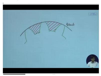
This is the original blank; this is the blank which means the material from which we are going to cut out some extra material, so that only that which is required remains. What is required? These are the teeth which are required, this is what is required. So, there is some material which is not required which can be quickly identified as this part. This has to be removed and it is on the milling machine that we do the removal of these tooth space material.
