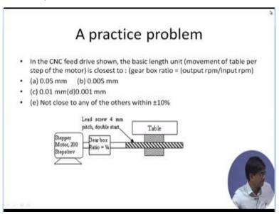
Another one slightly different configuration, but this will also help you to understand the application of gearboxes later on. In the CNC feed drive shown, the basic length unit that is the movement of the table per step of the motor. So, what do we have? We have a CNC system in which there is a stepper motor which rotates in steps to cover 1 rotation in 200 steps. So, 1 rotation is 360° and 200 steps are making up that one rotation.
