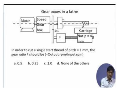
Have a look at this, the actual use of gearboxes in machine tools. First of all, why are we studying this? We are not supposed to become masters of gearbox calculations. No, but this would be required because we will be extensively using gearboxes and gearbox ratios, their calculations etc. in our, subsequent lectures. That is why 1 or 2 examples will really help.
