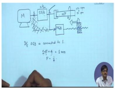
If I have a motor and then I am claiming that I have a speed gearbox here, from which I am rotating the workpiece. Now, you will find in the figure, we have taken a tapping from here and then I am putting another gear box called feed gear box. And then I am rotating something. On that, I have put a nut and moving it. Now, first of all, I could have connected it up here.
