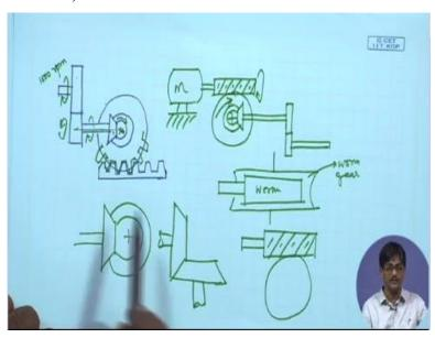
So, say here, we are having a gear connected with another one. So, let us see what sort of configuration that we are talking about. I might say that here, I am providing you 1000 RPM. These are spur gears. So, they are rotating say this way, this one is rotating that way. Now, this one, I wanted to introduce some typical figures, these are 2 bevel gears which are connected with each other.
