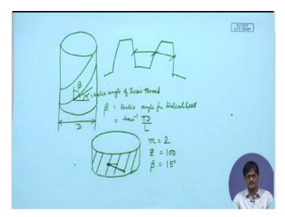
Suppose, these are helices on a screwed thread. In that case, we will express the helix angle as this one. And naturally if it is rising by p, in a single start thread, it will be:
