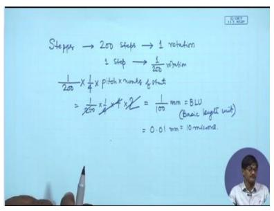
So, we have a stepper with 200 steps which gives 1 rotation. So, for 1 step we get  $\frac{1}{200}$  of a rotation. Therefore, I start with  $\frac{1}{200}$  of a rotation multiply it by the gearbox ratio one fourth multiply it with the lead screw lead; lead screw lead is Pitch into number of starts equal to  $\frac{1}{200}$  into  $\frac{1}{4}$  into pitches 4 millimetres and it is double start so, multiplied by 2 equal to  $\frac{1}{100}$  millimetres.
