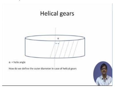
So, in case of helical gears, let us have a quick look at the depiction. The teeth are slightly inclined with respect to the central axis. So, we have drawn the central axis as a dot and dash line and the teeth are inclined at a particular angle  $\alpha$  which we are calling as the helix angle. Now, you will notice that when we are depicting the helix angle of screw threads and the helix angle of helical gears, they are complementary.
