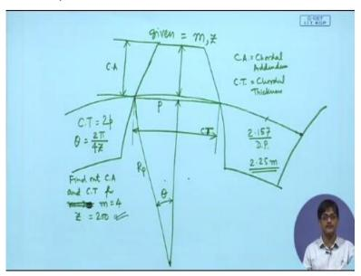
For example, you will find that in this figure if we make a larger depiction of this one, if this be one gear tooth, you will find that on the pitch diameter, we have depicted 2 dimensions. The bottom one being called as Chordal Thickness (CT). And this one being, which is joined by straight lines, this is equal to Chordal Addendum (CA).
