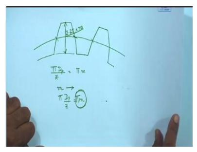
Let us take a fresh piece of paper if this be, how is module affecting its shape or size. We find that if we draw the pitch circumference from here to here, this distance is constant for all gears having same module. So, module defines this distance on all gears having the same module. So, this distance is equal to  $\frac{\pi \times D_p}{Z}$ . So, module is relevant to the gear teeth by this dimension.
