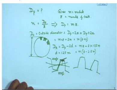
Pitch diameter has to be found out and what is given m = module; z = number of teeth. This is straightforward. We have the definition of module as:
