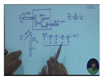
And if I tell you that make a gearbox into which it is moving in, put whatever ordinary gears that we have discussed up till now spur gears, I will come to this term spur gears, put whatever gears that you can put in and get me a speed of 10 RPM. So, you immediately find out what is the speed ratio required.
