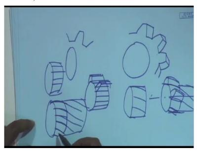
If you have a quick look here, I can have a gear of this type where the teeth are of this type as we have been drawing. That means if you look along the axis of the gear, the teeth are straight. So, that when you draw them, you can draw them this way, but you can also have gears in which the teeth instead of being straight. Here, we have drawn gears which are having straight teeth that means these teeth are this way.
