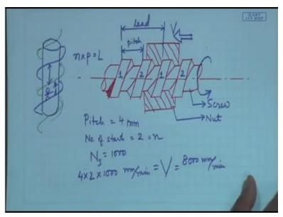
First of all, if you kindly have a look here, I draw an axis line to mean that whatever I am drawing it has its axis symmetric. And this is basically a screw, that is it. So, we have a screw to start with. So, it is basically a helix wrapped around a cylinder going this way. So, when you have such a member, it has a corresponding body called nut which can be fit on top of this.
